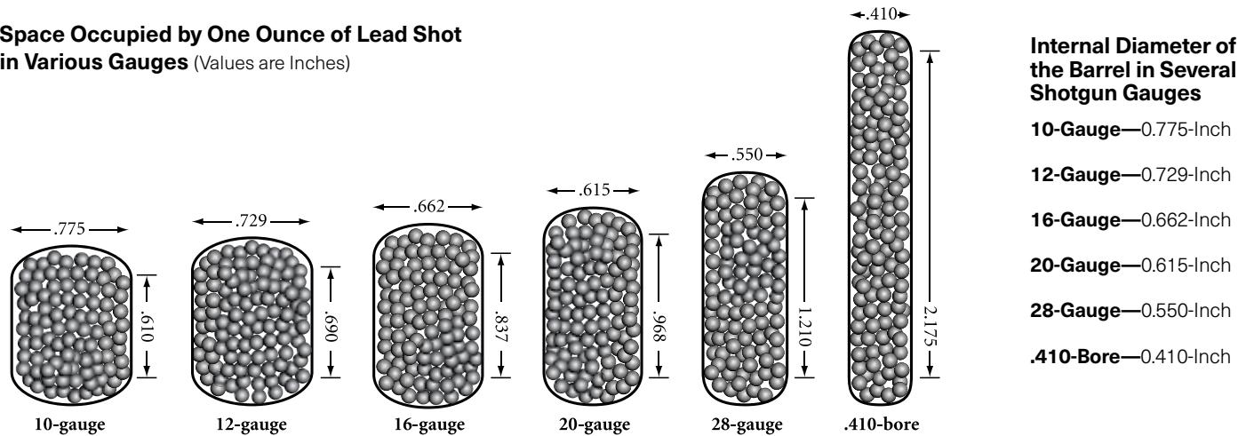
Internal Diameter of the Barrel in Several Shotgun Gauges
